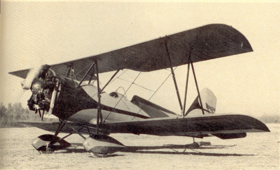
The larger diameter of the 160-hp Kinner engine in the OTW-160 ruled out the use of a cowling. This one has been dressed up with a postwar paint job and a set of wheel pants. Photo by author
